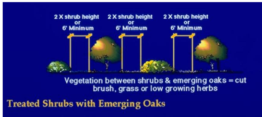
Figure 14. Shrub island spacing. Design groups of plants small enough to provide horizontal separation between groups. This allows proper maintenance and helps slow the spread of fire. Each shrub or group of plants should measure no wider than two times its height, or less than 120 sq. ft. (or 6 ft x 20 ft). The space between groups should be greater than three times the height of the shrubs.
