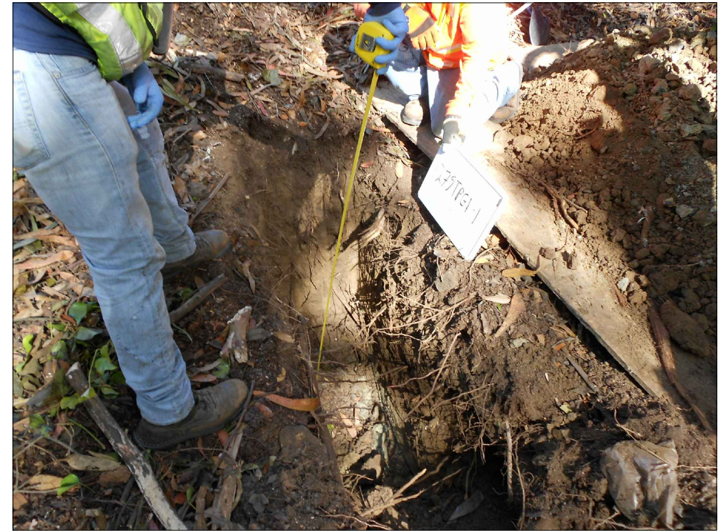
View into trench. Note degraded bedrock at bottom of trench.
