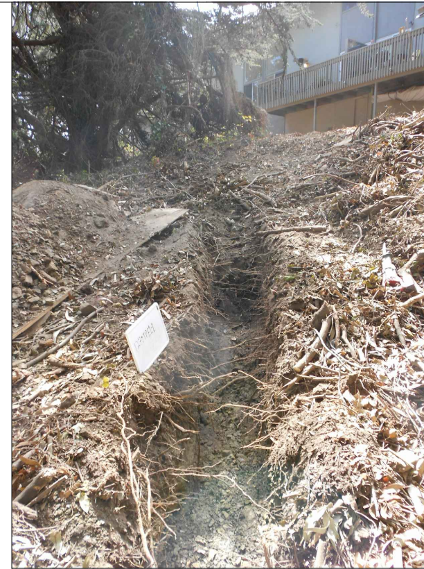
Area view along trench and portion of spoils pile. Note ash at far end of trench and in spoils pile (uphill) decreases to the northeast (downhill). Note large cypress tree in background.
