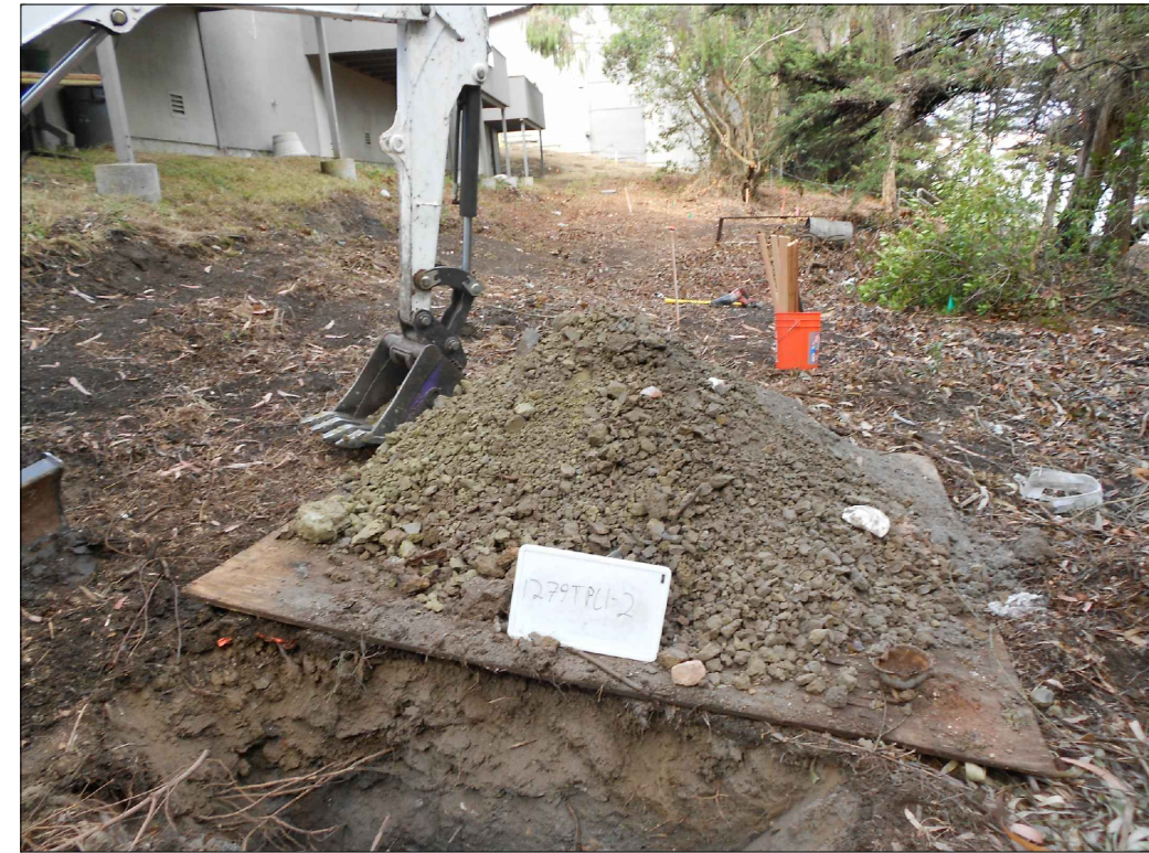
Area view of trench and spoils pile. Note change in color of spoils, with native on left and ash to right rear of pile.
