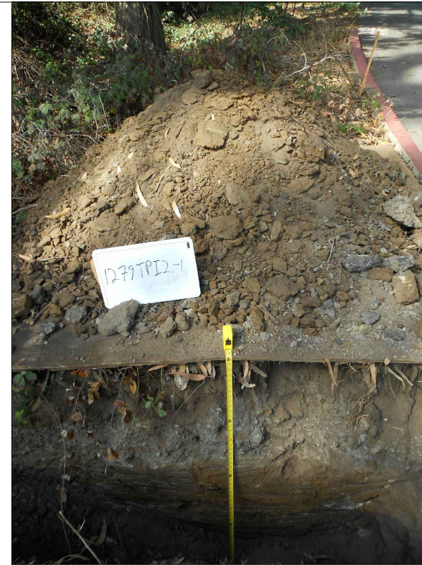
Spoils pile. Note cobbles and asphalt in spoils.
