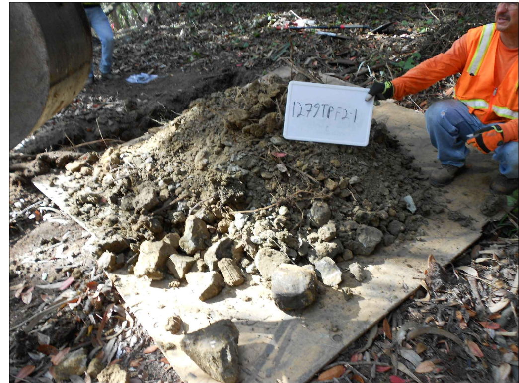
Spoils pile. Note large cobbles from shallow surface and debris layer.
