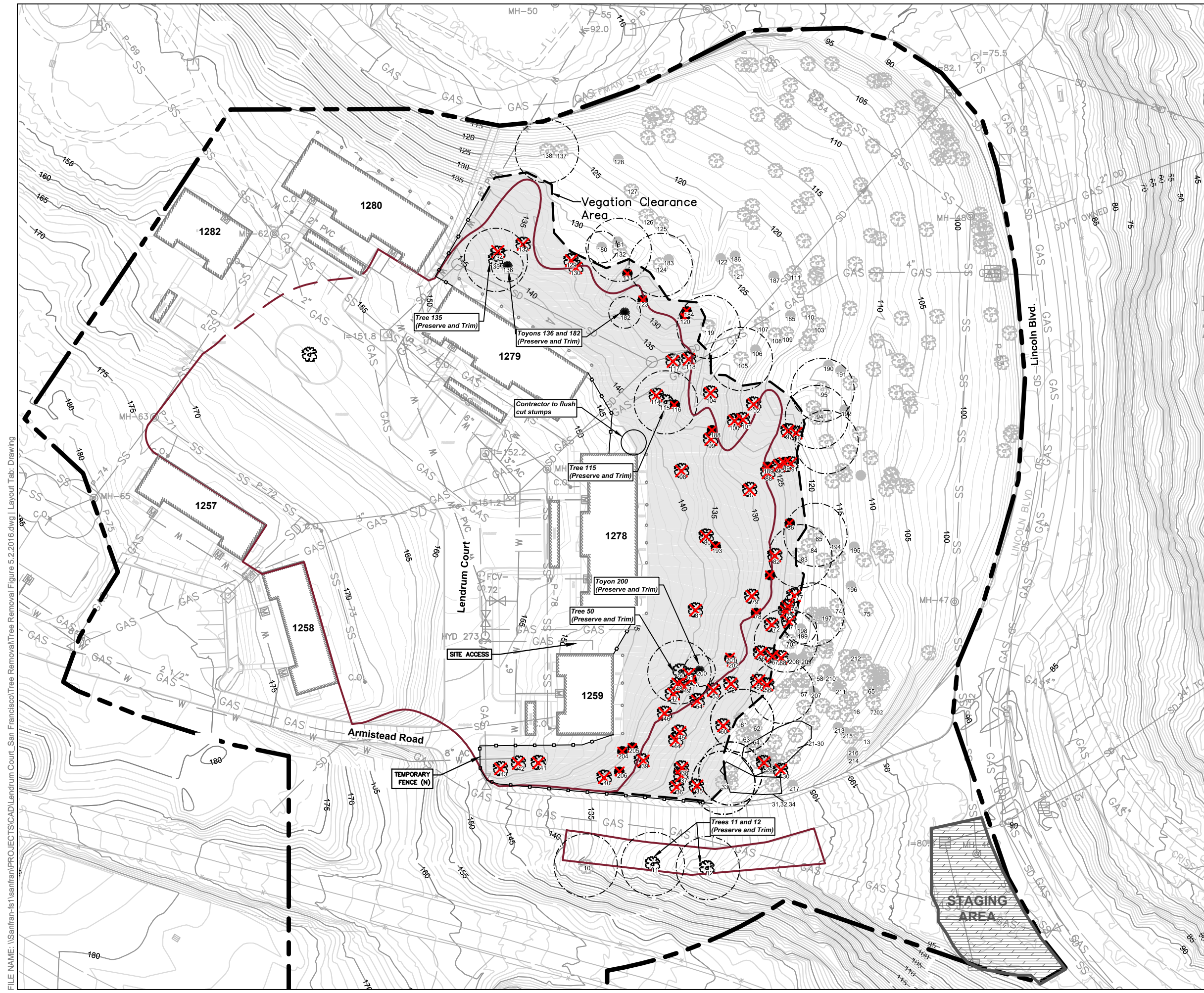
Figure I-2 Tree Removal Plan
