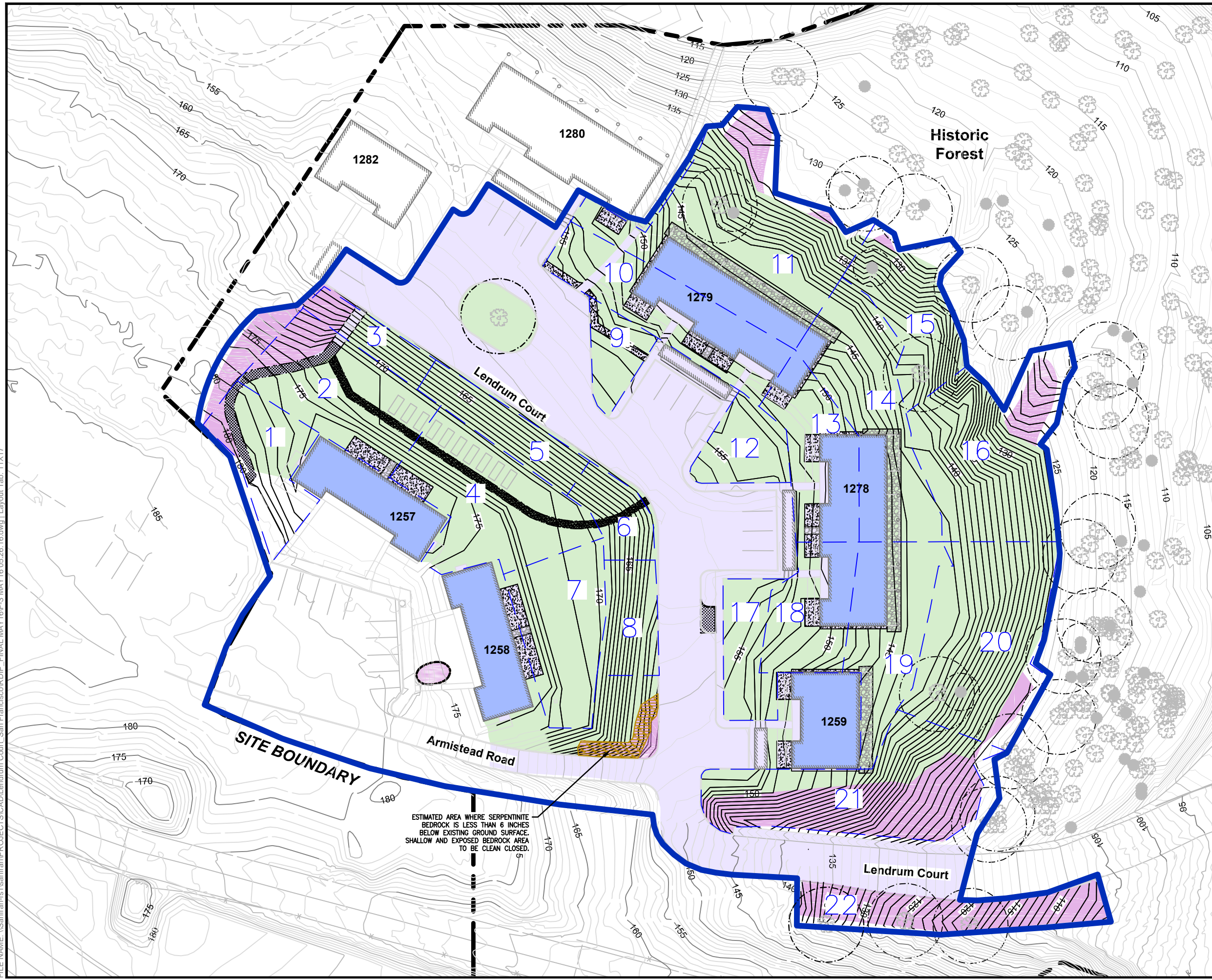
FINAL GRADE- PROPOSED LOCATIONS FOR SOIL COMPACTION TESTING May 26, 2016 Lendrum Court Area The Presidio Trust San Francisco, California
